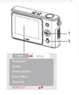
Press OK/Enter on the five-way control button (1) to save the settings and finally press the MENU button (2) to close the menu
